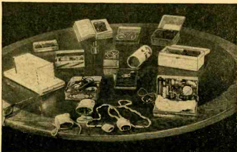
Mr. Maquerinck was unable to take photos of his radios. These underground sets were described in an article in the Philips Technisch Tijdschrift.
